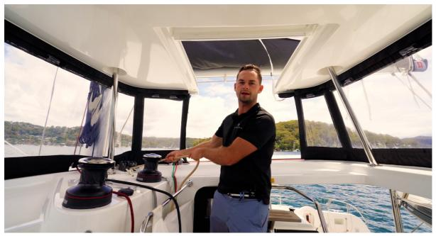
Make sure all the slack on the mainsheet is pulled in just to stop the boom swinging around too much if you are in a bit of swell.
